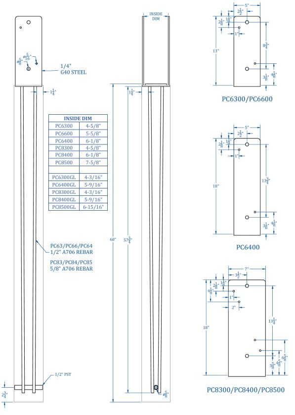
Figure 4.2 Structural Reinforcing Bracket Assemblies
