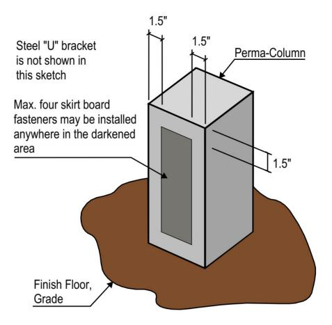
Figure 9: Placement of skirt board fasteners
