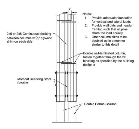
Figure 7.1 Double *Perma-Column* installation detail
