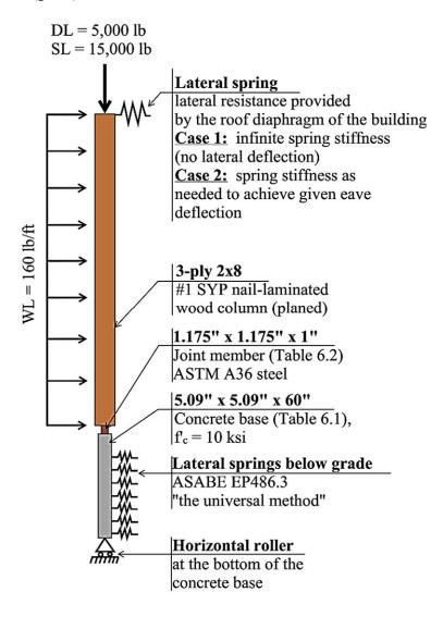
Figure 8.1 Structural analog for Design Example
