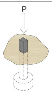
The calculations are completed using the Load Resistance and Factor Design (LRFD) consistent with the ACI 318 adopted method, and the results are presented in terms of the Design Axial Strength. The Design Axial Strength in the calculations below is also converted to the Allowable Axial Strength using the conversion factor  $\alpha = 1/1.6 = 0.625$ . The calculations are completed in Microsoft Excel (2016) using the listed equations.
