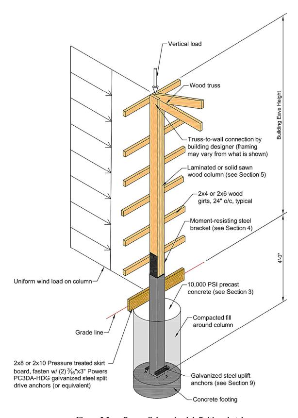
Figure 2.2 Perma-Column load definition sketch
