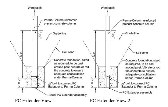
Figure 11.2: Foundation with PC Extender
