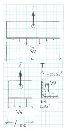
(6) The design tensile strength and the allowable tensile strength, as defined by the bending strength of the steel angles, is determined as follows:  $\phi T_n = \phi M_n / x$ ,  $T_n / \Omega = (M_n / \Omega) / x$
