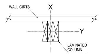
Figure 2.1 Wood Column Orientation
