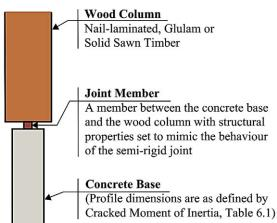
Figure 6.3 *Joint Member* between concrete base and wood column
