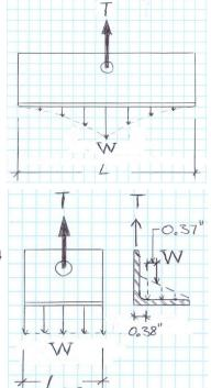
(6) The design tensile strength and the allowable tensile strength, as defined by the bending strength of the steel angles, is determined as follows:  $\phi T_n = \phi M_n / x$ ,  $T_n/\Omega = (M_n / \Omega) / x$
